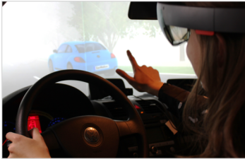
Investigation of augmented reality (AR) timing constraints in a driving simulator environment.
